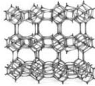
Figure 4. Zeolite structure (Source: International Zeolite Association).
