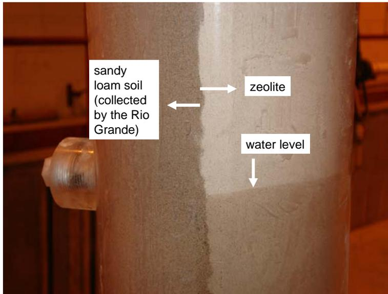
Figure 5. Split test of fine clinoptilolite and sandy loam soil in 4-in acrylic pipe.
