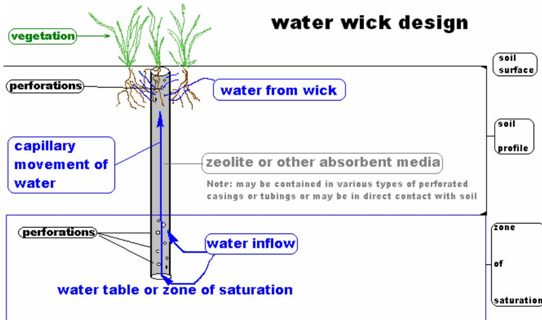
Figure 3. A schematic of the water wick method using clinoptilolite.
