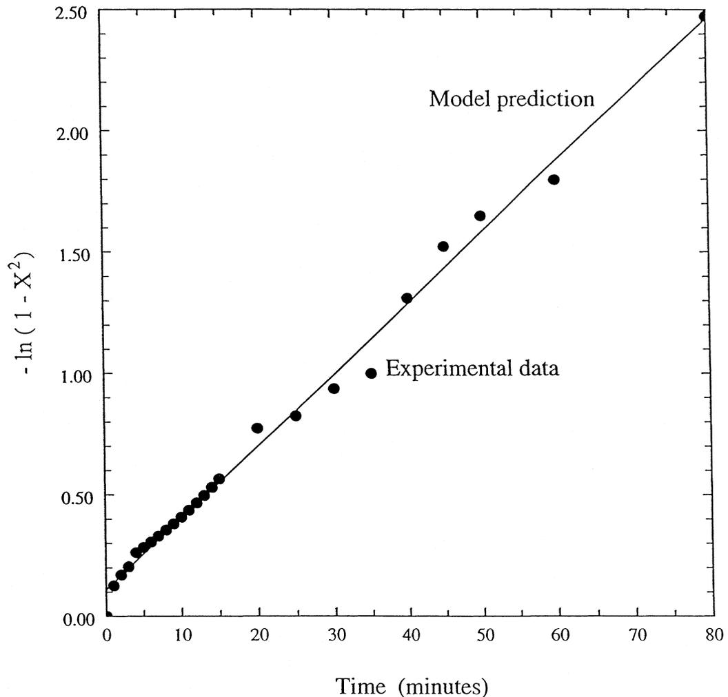
FIG. 3 Rate test results applied to Vermeulen's approximation. Ammonium adsorption onto Na-form zeolite. Initial solution concentration 50 mg  $\text{NH}_4\text{-N/L}$ . Zeolite size range 425 to 600  $\mu\text{m}$ .
