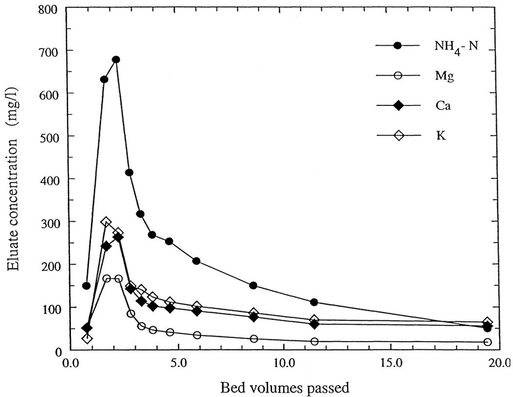
FIG. 6 Typical elution profiles for NH<sub>4</sub><sup>+</sup> and competing cations. Regenerant is 0.6 M NaCl at pH 10.
